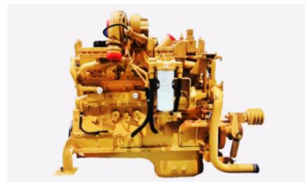
Cummins Country III engine, add intercooling CAC, optimization Fuel supply system to improve fuel efficiency and improve mobility More powerful, reliable and environmentally friendly;
